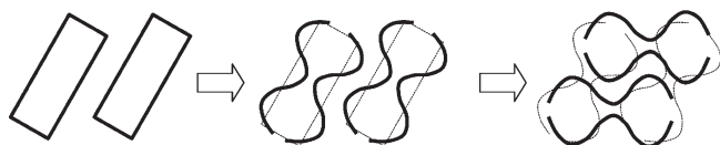
Figure 5. Possible structural transition mechanism from randomly oriented LAM to epitaxial HML.
